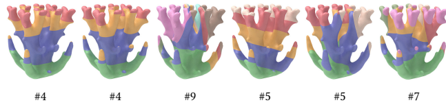
Fig. 12. Single variable comparison of each evaluation criterion, where we evaluate the generated blocks with only considering one of the six criteria. From left to right, this figure shows the decomposition results of (1) "Size of block"; (2) "Surface point priority"; (3) "Block connectivity"; (4) "Changing in print directions"; (5) "Structure soundness"; (6) "Pyramid-like shapes". The number of resulting blocks is indicated in the figure.
