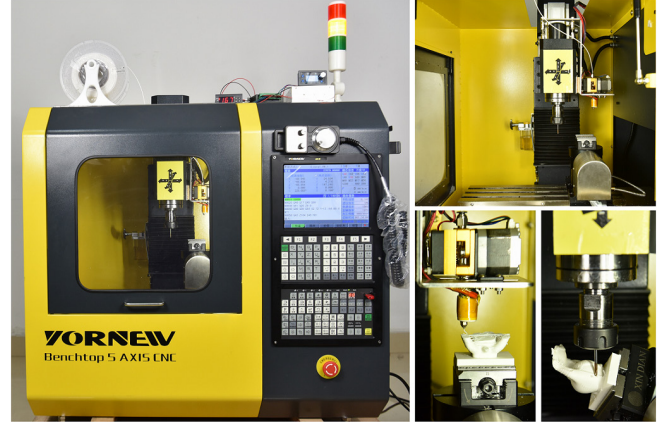
Fig. 19. Our ASHM machine was modified from a CNC machine (YORNEW Benchtop 5 Axis CNC MX220). The accessories of the additive module are installed above the machine (left). The additive extrusion module is connected with the machine spindle in parallel (upper right). The lower right corner demonstrates the additive process and subtractive process.
